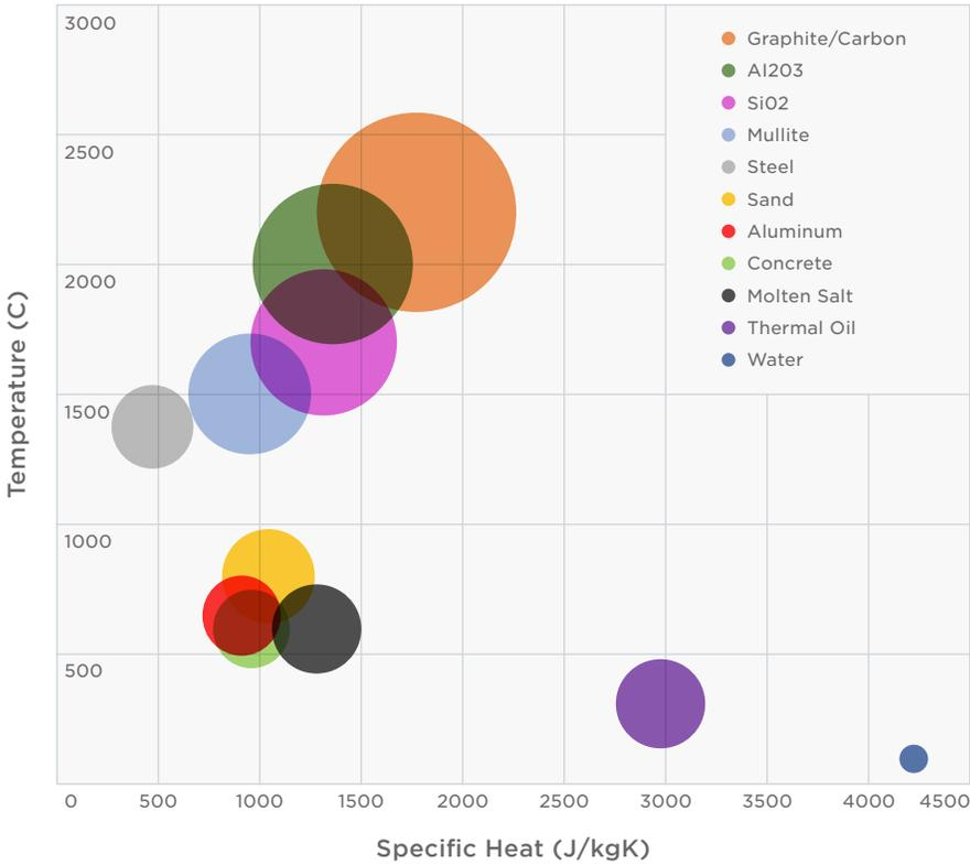
Figure 10: Thermal Storage - Heat Storage Media
