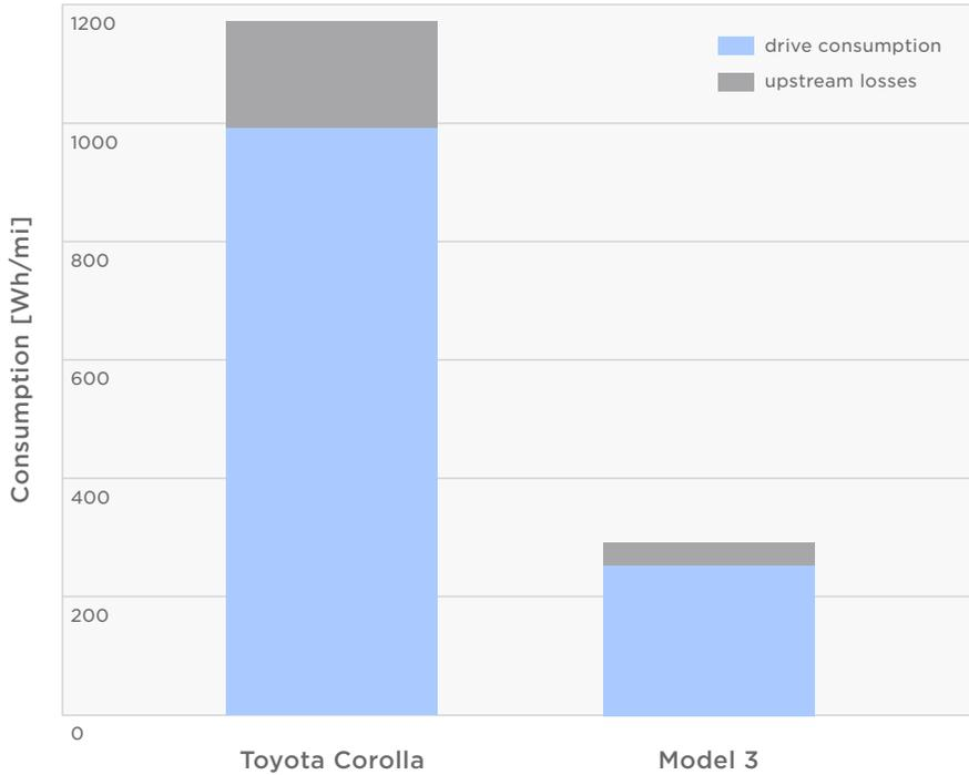
Figure 4: Comparison Tesla Model 3 vs. Toyota Corolla
