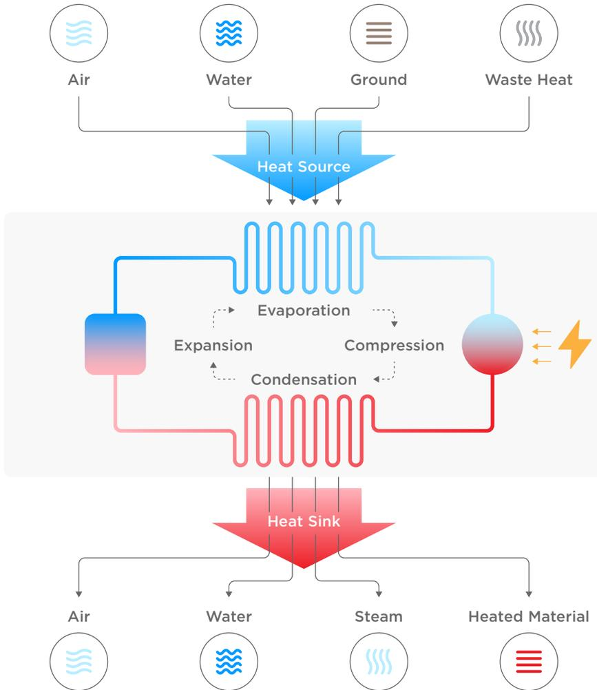
Figure 5: How Heat Pumps Work<sup>10</sup>
