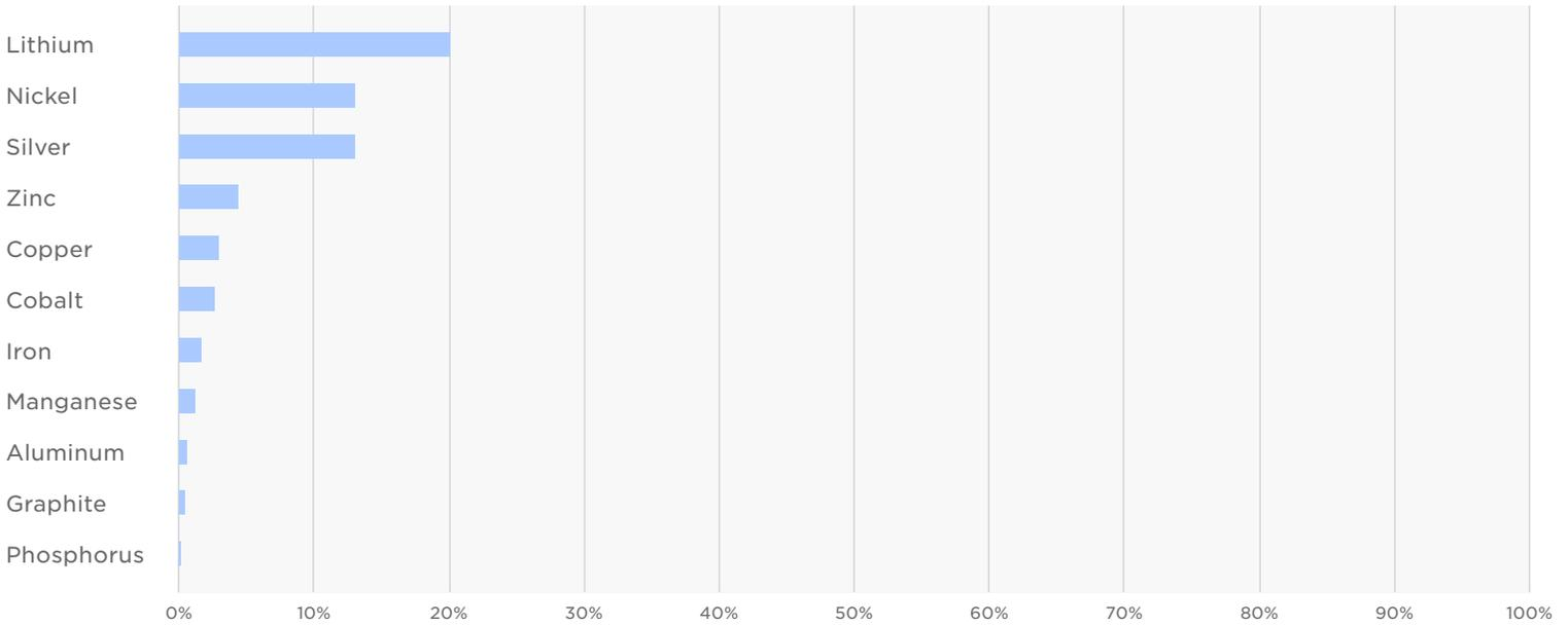
Figure 17: Materials Required Relative to 2023 USGS Estimated Resources
